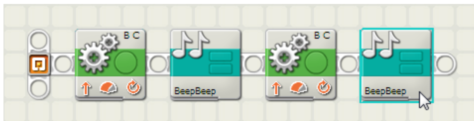
Figure 11: My Blocks can be easily re-used, saving both programming time and memory on the NXT.
